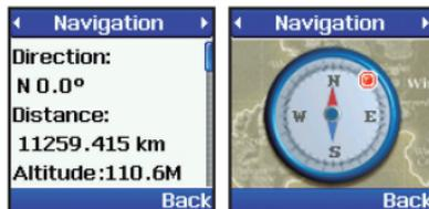
Numerical and directional information can be checked using
